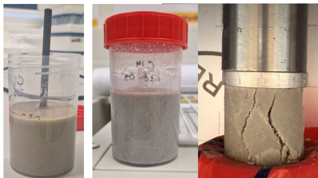
Fig. 1. Preparation of the sand-silica gel samples for gelation time and mechanical test measurements.
