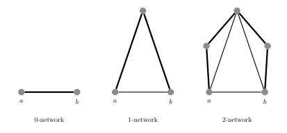
Consider following iterative construction: A 0-network consist of two initial vertices a and b connected with a link. Iteratively, an (n + 1)-network is obtained from the n-network by glueing a triangle to each newly added link at the previous iteration, as shown.
